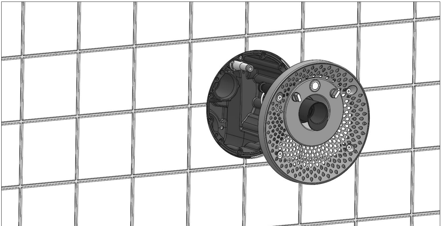
Fig. 26 Attach the nozzle head (note position of the pressure connection and air connection) and screw it on.
